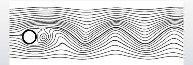
Frequency of vortex shedding near to Frequency of acoustic resonance
